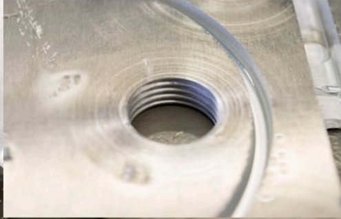
a thread tap (used in the heater) simplifies the shape but complicates the construction
